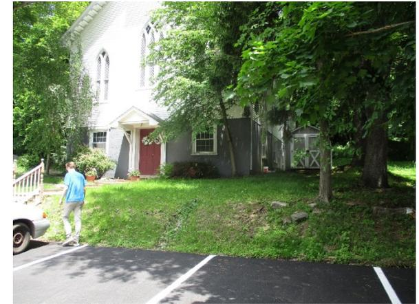
A rain garden can be installed in the turfgrass area on each side of the entrance to capture stormwater from the downspout. Pervious pavement can be installed in the parking spaces to intercept stormwater from the parking lot. A preliminary soil assessment suggests that more soil testing would be required before determining the soil's suitability for green infrastructure.
