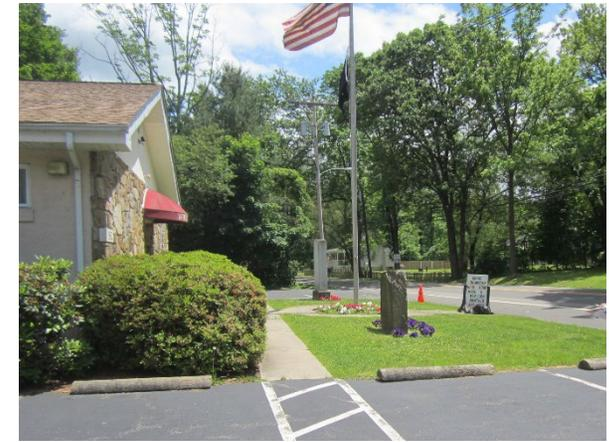
A rain garden can be installed on either side of the entrance to capture stormwater from the rooftop by redirecting the downspout under the sidewalk. Pervious pavement can replace sections of parking spaces to capture a large portion of the parking lot runoff. A preliminary soil assessment suggests that more soil testing would be required before determining the soil's suitability for green infrastructure.
