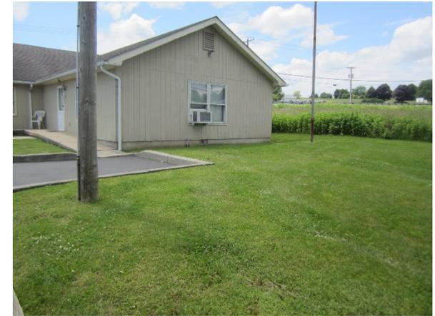
A rain garden can be installed in the turfgrass area northwest of the building to capture stormwater from the rooftop of the building. A preliminary soil assessment suggests that the soils have suitable drainage characteristics for green infrastructure.
